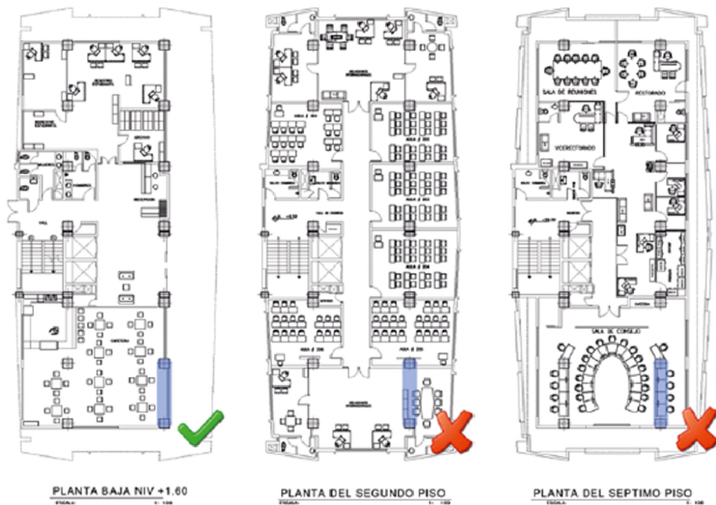
Figure 5.28 Difficulties in finding an appropriate location of a new shear wall: a valid location in one floor blocks the operation of other floors. Source: Stelios Antoniou.
